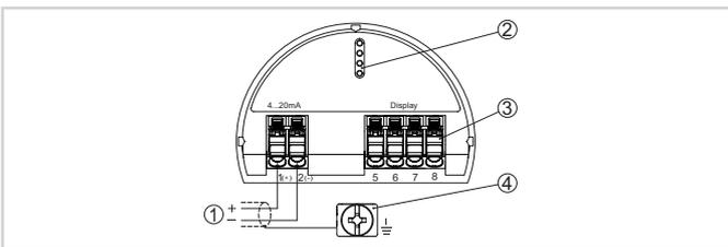
Electronics and connection compartment, single chamber housing (example)
